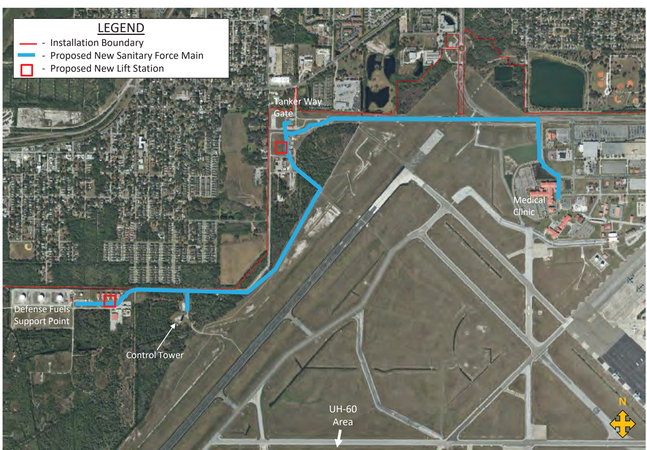
Figure 2: Location of proposed force main piping for the Northern Route Alternative considered for expansion of the sanitary sewer system to the western side of the installation.
